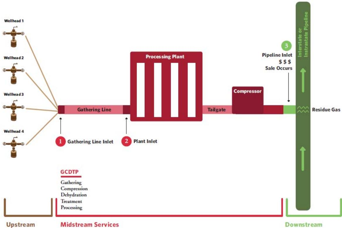
40. As the gaseous mixture from each well enters the gathering line, it flows into a meter run where the mixture is measured for both volume (in Mcf) and quality (Btu content) (combined, “gas measurement,” in MMBtu). The meter run must be constantly maintained to record accurate measurements.
